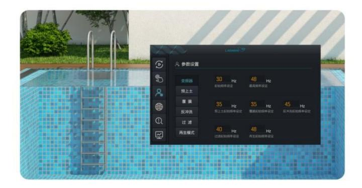
Equipped with a PLC smart control system, the unit automatically switches between precoat, filtration and regeneration modes, ensuring user-friendly operation and efficient performance.
