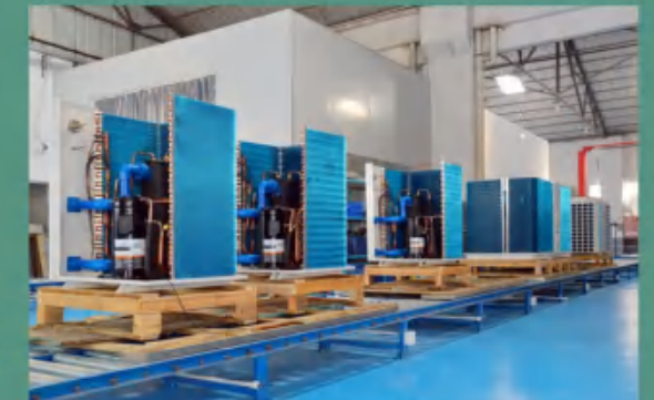
Heat pump production workshop
