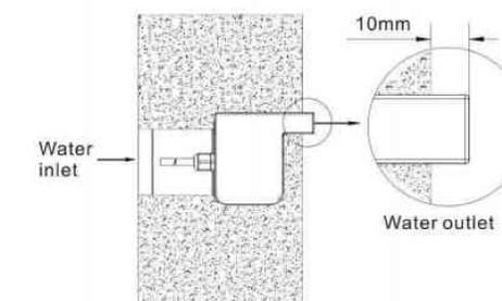
Installation for piping single unit with ball valve
