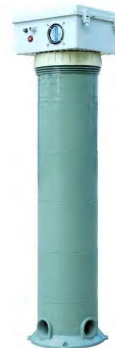
Specially designed for sea water environment. The housing is made of high quality PVC, which is anti-corrosion and durable. Equipped with UV-C lamp and high purity quartz sleeves for high efficient and long term sterilization. The disinfection process is fully closed, with sound and light alarm device, no chemical reaction and by-products.
